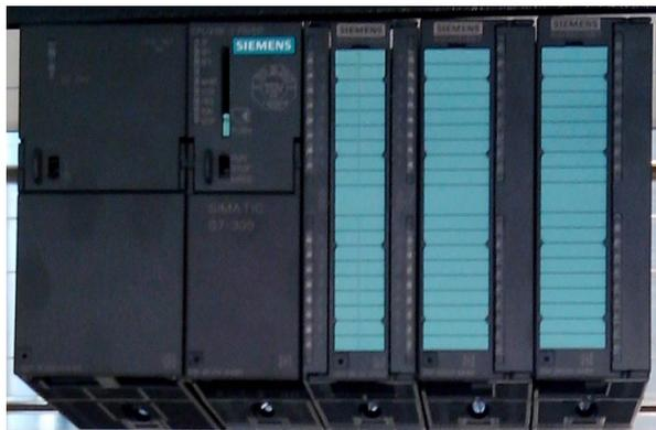
Figura 2.7: CLP Siemens - Simatic 300.
