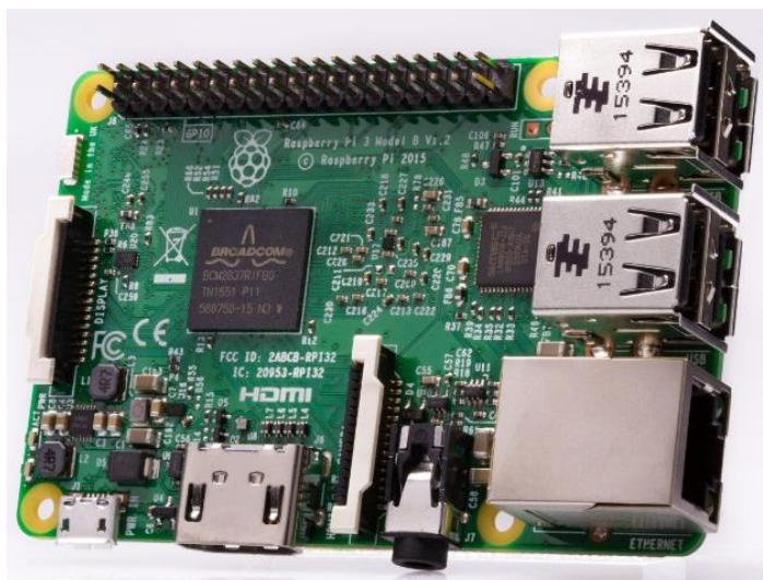
Figura 16 - Raspberry Pi 3 Model B.
