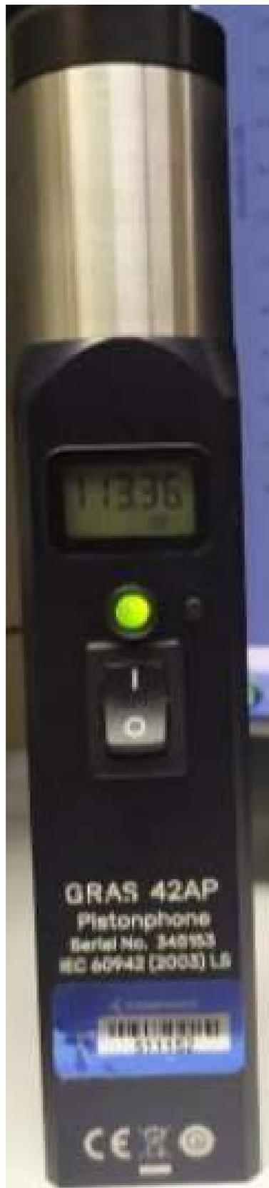
Figura A.3: Pistonphone da *G.R.A.S Sound and Vibration*, modelo 42AP
