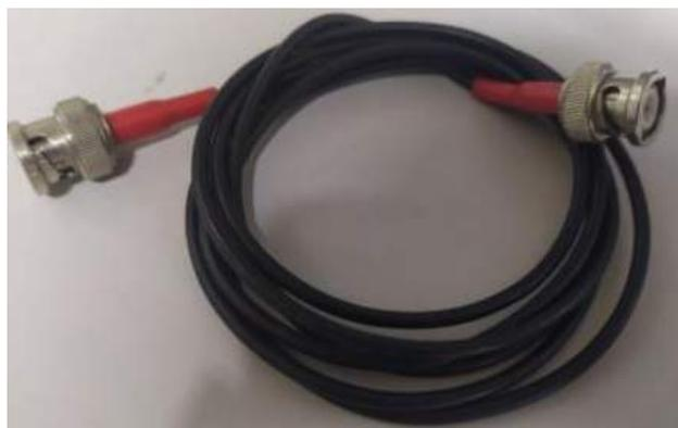
Figura A.12: Cabos BNC-BNC
